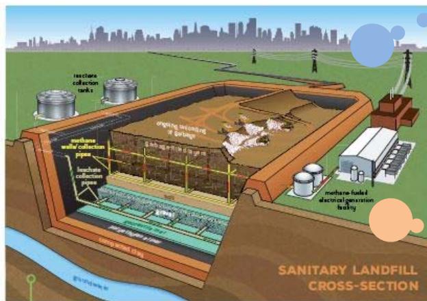
Sanitary landfills vary in size and depth. But most have a thick clay lining on the bottom and sides, several layers of absorbent substances on the bottom, and pipes for transporting liquid to the surface. Some landfills include pipes that collect methane for power generation.
