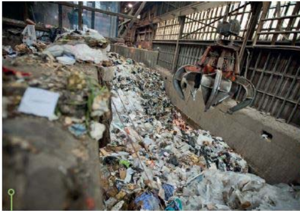
Many US cities dispose of garbage by burning it in big incinerators. At this incinerator in Harrisburg, Pennsylvania, a mechanical claw grabs garbage and moves it to a furnace.
